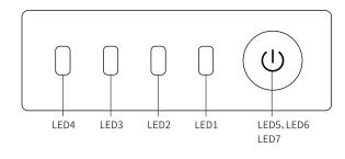
LED1, LED2, LED3, LED4 are green lights and show the battery SOC and lifespan(SOH) LED5, LED6, LED7 are red, orange, and green lights to show the working status and warning information
